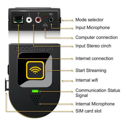
The **DIGOSTREAM Portable Link** allows quick and efficient streaming of the audio to the Internet via the DIGOBIT Stream Server.
